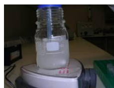
When aliquoting, use a stirring platform and magnetic stir bar to keep the beads evenly suspended
